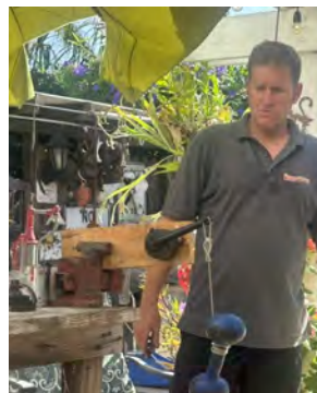
Testing shock with 15 lb. weight. Should take 6-7 seconds to travel to bottom of stroke.
