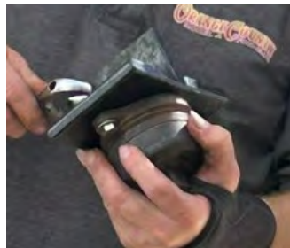
Mount shock base to holding fixture, before clamping in sturdy vice.
